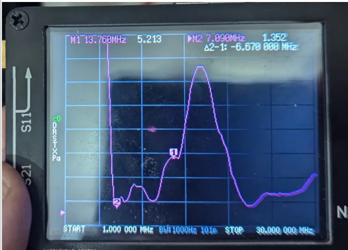
The tuner created a few dips, one on the 40 meter band
