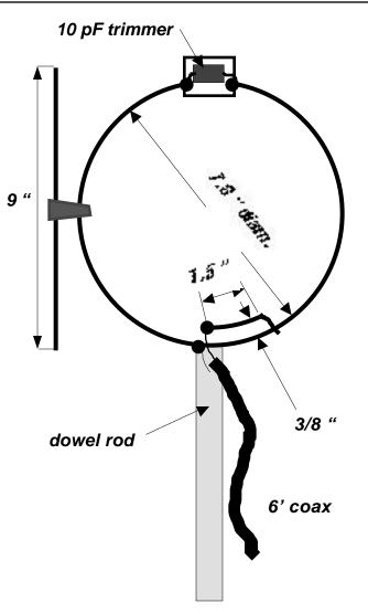
Use the maximum lobe to locate the fox when the signal is weak. Then when the signal is strong, use the nulls that are perpendicular to the plane of the loop to home in on him! This project shouldn't take more than 2 or 3 hours. Good luck and good hunting!
