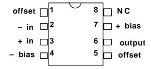
The connections to pins #2, #3, and #6 are self-explanatory, since these are the inverting input, the non-inverting input and the output, respectively, and they always appear in circuit diagrams. The two dc bias connections do not usually show up in circuit diagrams however. The dc power supply to the chip must be connected to these pins. The 741 requires a bipolar (both polarities) supply ranging from about 9V up to 15V. A typical hook-up using 9V batteries is illustrated below:
