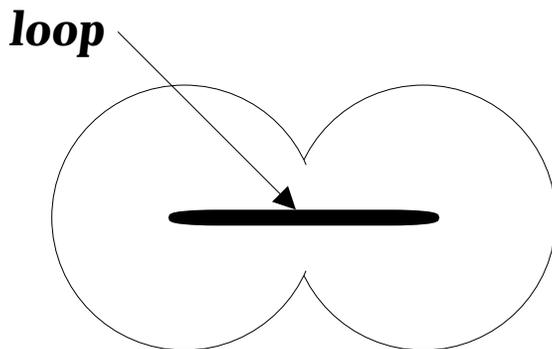
In other words, the maximum signal strength is detected when the transmitter is located off to the side of the loop. As you can see, the loop doesn't distinguish whether the source is to the right or to the left. This ambiguity in direction is not good enough for serious fox hunting!
