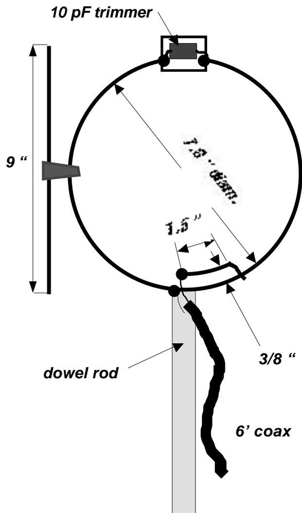
Use the maximum lobe to locate the fox when the signal is weak. Then when the signal is strong, use the nulls that are perpendicular to the plane of the loop to home in on him! This project shouldn't take more than 2 or 3 hours. Good luck and good hunting! ■
