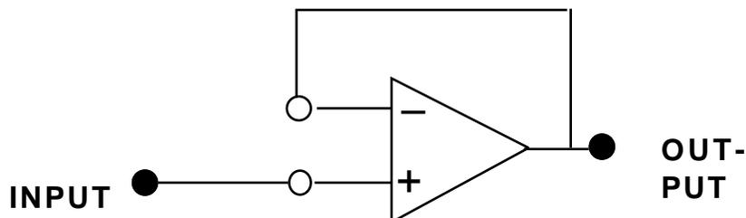
According to the formula above for the non-inverting amp, this circuit has a gain of one! What possible use is an amplifier that only repeats the input signal at the output? The answer lies in the input impedance, which can be on the order of 100's or 1000's of Megohms. This circuit provides a perfect *buffer* between a high impedance source like a crystal mike and a low input impedance amplifier stage. *next week - adding and subtracting* ■
